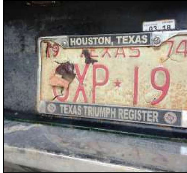
What 13 days of flood water does to a restored license plate – from Len and Marti Myers' totally submerged TR6 now restored
